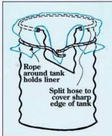
Steel tank without lid.
